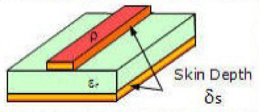
As frequencies increase, conduction begins to move from an equal distribution through the conductor cross
