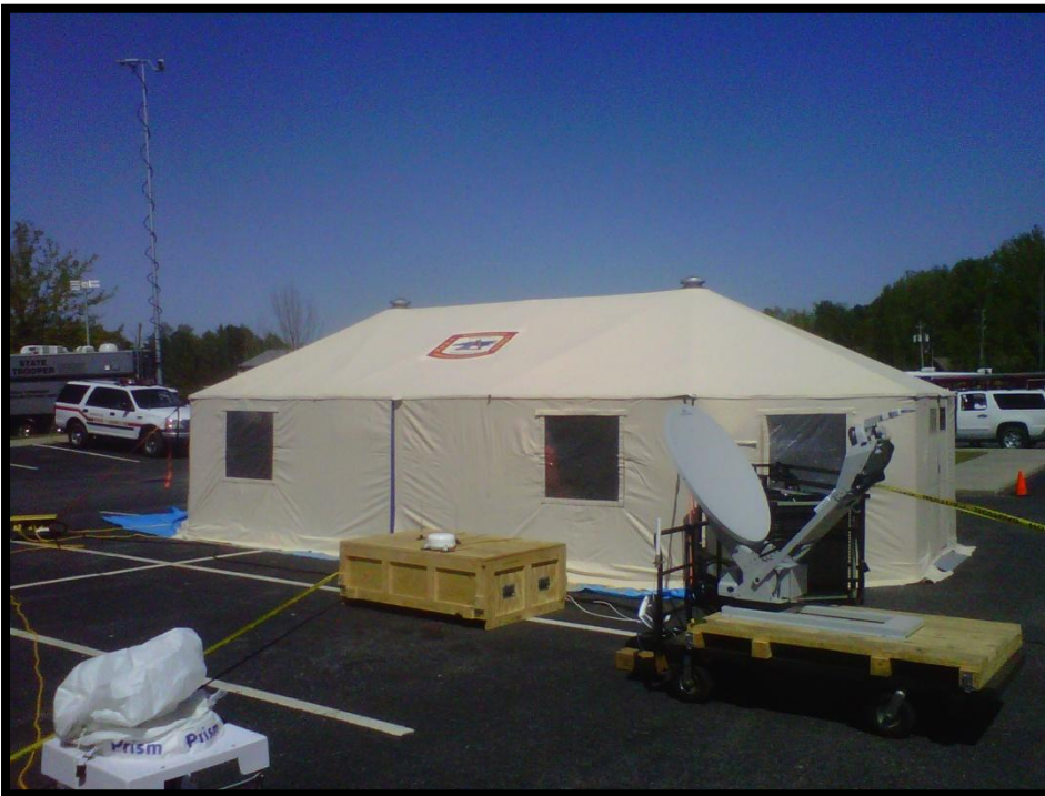
Outside of main BoO tent with comms. VSAT, MSAT antennas pictured. Note safety area around antennas.
