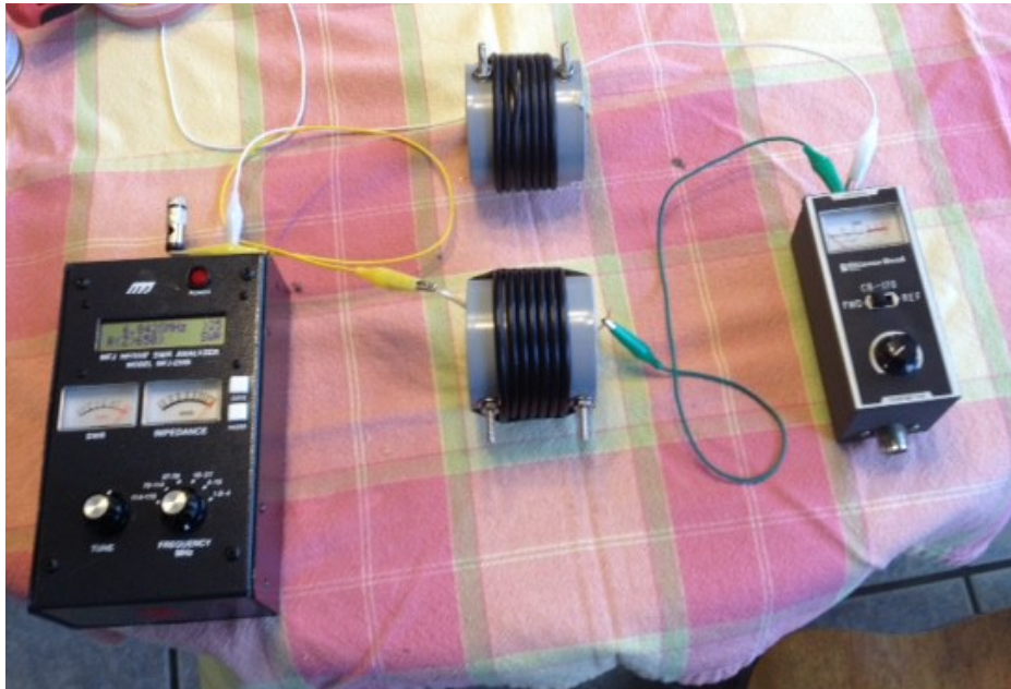
Homemade coaxial cable traps under test to determine their center frequency..
