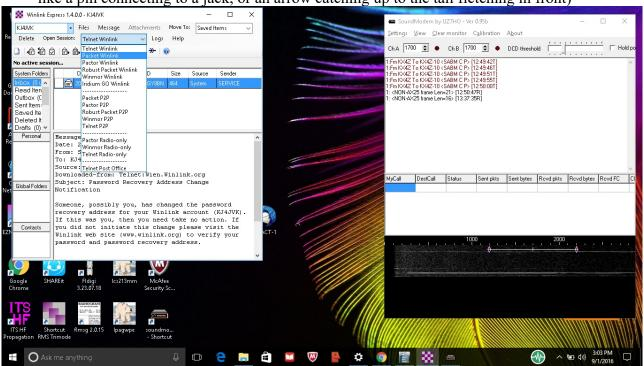
13. **Settings:** Once you have the Session dialog open, you may wish to check the **SETTING** to verify that it is correctly set for **KISS TNC** (provided in software by UZ7HO soundmodem.exe) and using TCP connections on 127.0.0.1 (your computer's "myself" address, on the exact same port (8100) that the soundmodem.exe software is expecting you to be on. Speed is 1200 baud, **MAXFRAMES=1** and the **packet length** may be either 64 or 128.
