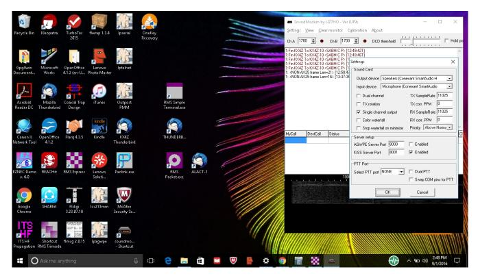
5. Check the **Setting** | **Devices** that the audio is going to the SIGNALINK and not to the computer mic and speakers – the connected devices for output and input should include the word "USB".
