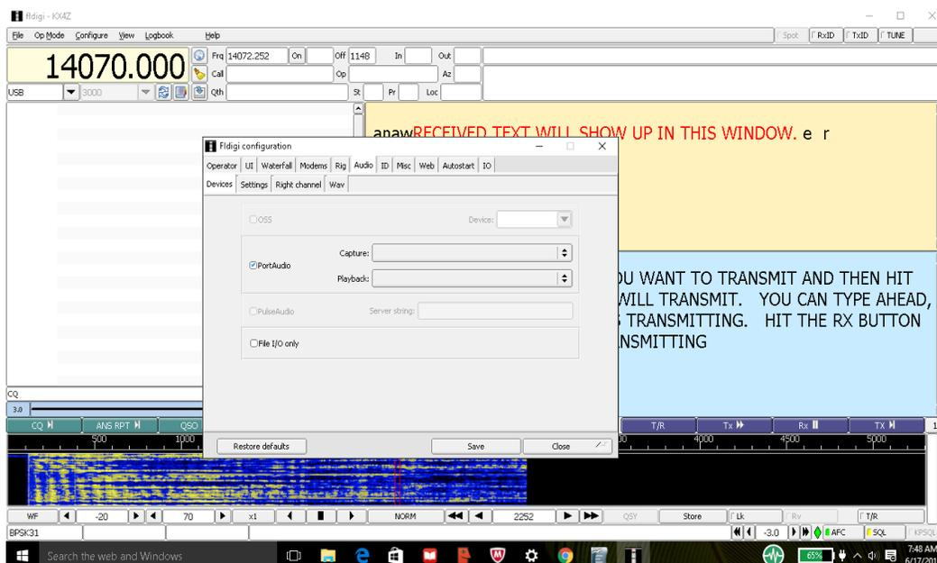
For Signalink, you will want to choose both for input and output-- SOMETHING that has “USB” in its name – the giveaway that the device is your Signalink device. You can ONLY have ONE signalink on a given computer, so don't try using 2 for some reason....
