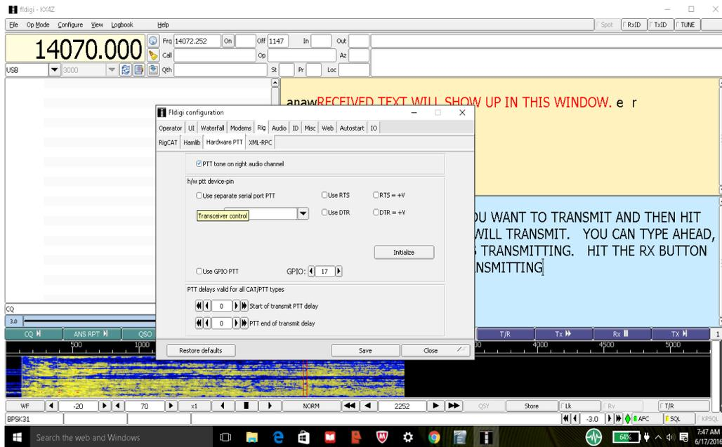
For Signalink devices, a continuous tone is sent on the RIGHT channel of the audio system which activates circuitry to invoke the Push To Talk. Your audio volume on the computer right channel needs to be at 100% If you are using some form of serial port controlled push to talk, you will need to configure it here.
