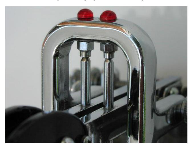
The frictionless two-point suspension is used, e.g., in the Vibroplex Racers, the ubiquitous Bencher, the G4ZPY. This construction is best visible in a close up of the Hamco Scotia (seems it has grown some moss in the past 25 years...):
