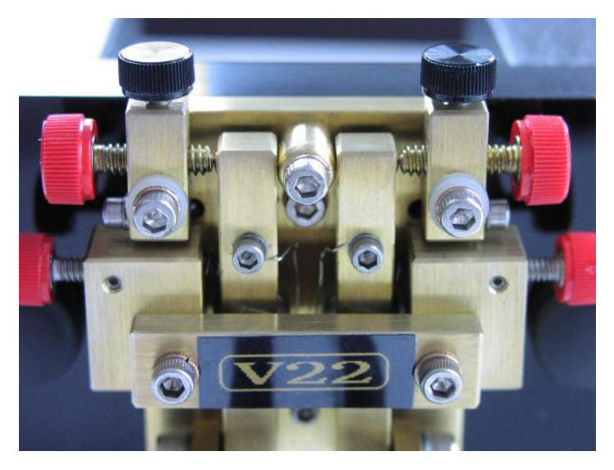
Earlier than most makers he realized the importance of minimizing the moving masses in a key by reducing the component size, and he maintained the ideal leverage ratio by opting for a vertical architecture. By bending the levers at a sharp angle at the bottom, the two sides of the lever can be made about the same length (1:1 leverage) despite the diminutive size of the mechanism.
