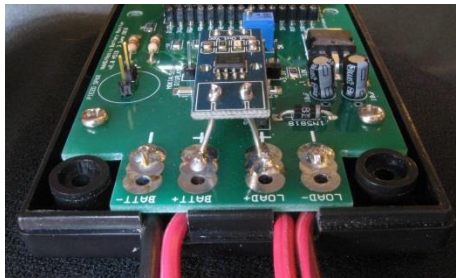
Figure 15. Additional views of populated PC board, including piezo speaker connected
