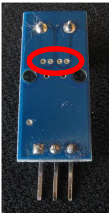
Figure 10. Vias joining top and bottom side traces
