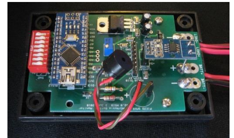
Figure 15. Additional views of populated PC board, including piezo speaker connected
