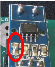
Figure 9. Filter capacitor on current sensor module
