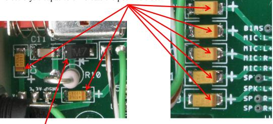
The polarity protection diode, a 1N4007, marked "M7" has a grey striped bar that identifies its cathode (-) terminal.
