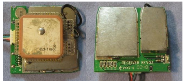
Figure 4. GPS receiver module, top and bottom views
