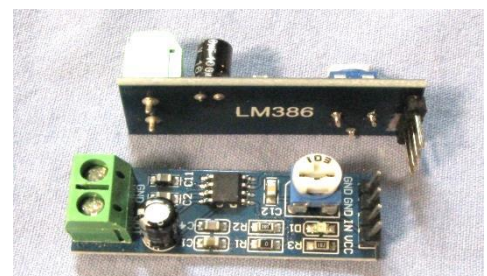
Figure 8. LM386 audio amplifier modules. With factory pins (bottom), and modified pins (top)
