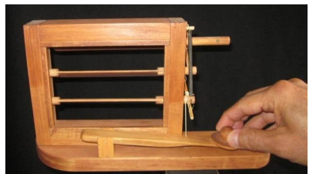
Morse key pressed, shutter OPEN
