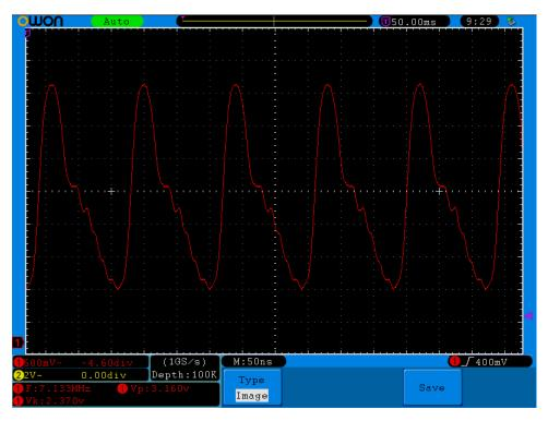
This next 'scope trace shows the output of the power amplifier and low pass filter, taken across a 50 ohm resistive dummy load. The nice 38.6 Vpp sine wave allows a calculation of the output power as approximately 3.7 watts. Thus the gain of the final stage is about 17 dB! Power supply voltage, measured on the PCB, was 12.5 V, and total current draw was 630 mA (~ 50 mA for the TT2 portion) for about 50% efficiency of the PA.
