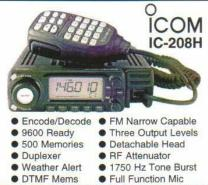
The ICOM IC-208H 2M/440 dual bander features: detachable control panel, wideband receive, CTCSS decode/encode, PC compatibility and 500 alpha memory channels. Output is 55/15/5 watts on 2 meters and 50/15/5 watts on 440 MHz. The 208H also includes a built-in duplexer, packet port, OPC-600/R separation cable, HM-133 remote hand mic, mobile mounting bracket and spare fuses. Requires 13.8 VDC at 12 amps. List \$396.00 Order #0208 \$289.99 [Price shown is after \$20 Icom mail-in rebate]
