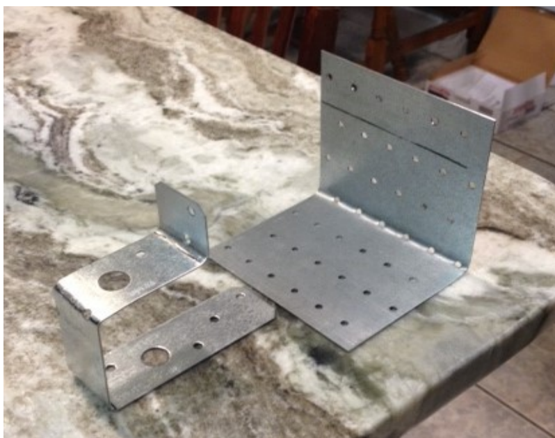
Hand-Bent Brackets – using vise, table edge and small hammer
