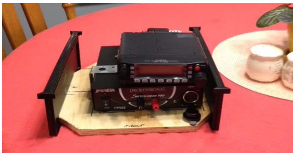
AC power supply and radio assembled on plywood base attached to plastic RIDGID box dividers so system can be inserted and removed.
