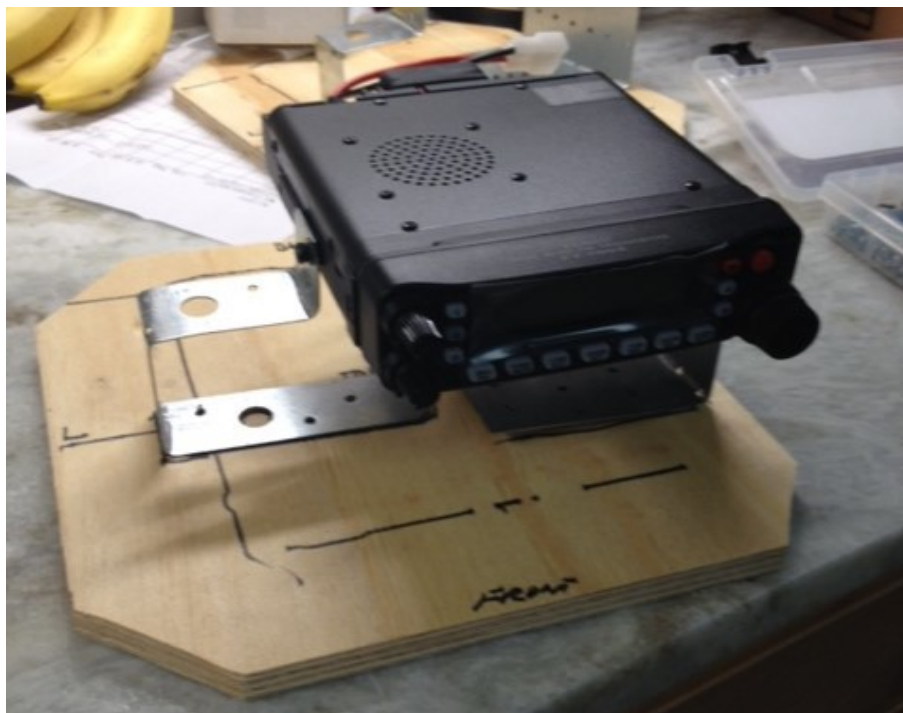
Marking the screw hole locations for the left bracket.
