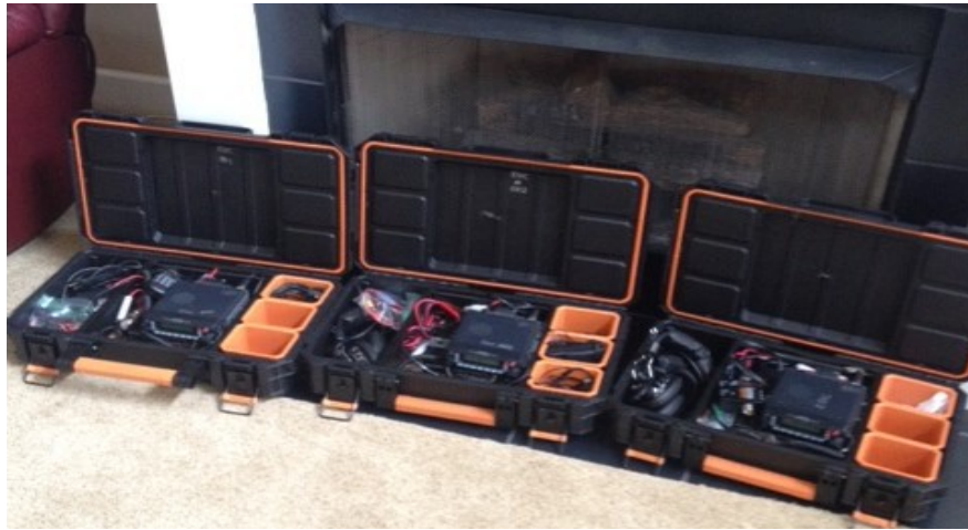
Three VHF transceiver go-boxes constructed by Alachua County ARES volunteers in time for Hurricane Irma
