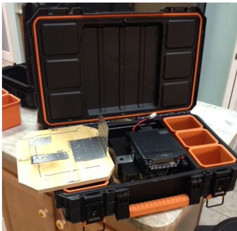
Comparison of finished radio mounting and in-process plywood base with brackets.
