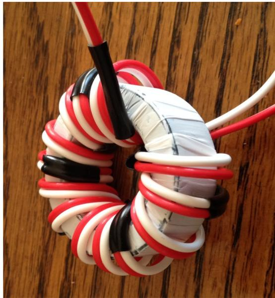
In this photo the toroid has been wrapped with teflon tape (the kind plumbers use for pipe fittings) to protect the teflon insulated wire and the wires kept close together with some insulating tape --- some designs run them inside a plastic tube; others use 2-conductor speaker wire.
