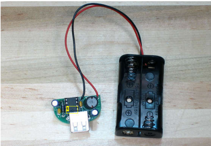
Image Notes 1. Insert the chip so the notch is over here, like the socket
