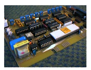
The TCX 150G Repeater Controller runs on a 486 PC in DOS and supports five ports, voice id's, announcements, weather status, cw id's, rotatable id's and announcements, 40 tail tones, 4 kinds of autopatch with tone regeneration. All sounds are easily modified way files so you can record your own files.
