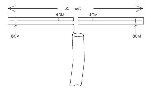
I'm sure that somebody will build one of these for LOCAL 160M / 80M operating. I say local because it must be close to the ground in terms of wavelength (and therefore radiation is straight up). Just double the above dimensions.
