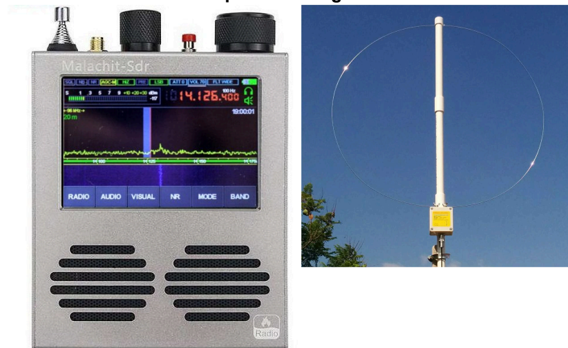
Figure 2.5: Malachite v1.3 DSP Receiver connected to K-180WLA —Receive-only Magnetic Loop antenna (MLA)
