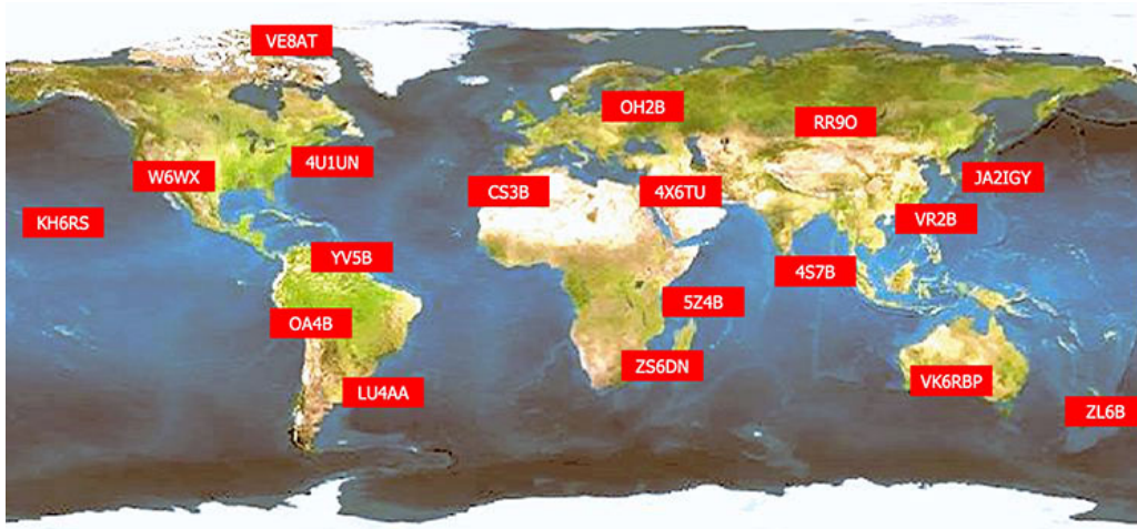
Figure 2.7: NCDXF beacons map —All use standardized antennas and power levels.
