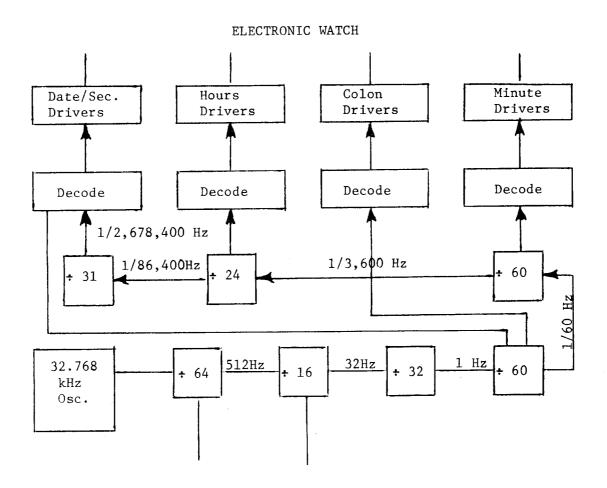
Start with a 32.768 kHz crystal oscillator. Use a divider chain to divide by 64 = 512 Hz  $\rightarrow$  divide by 16 = 32 Hz  $\rightarrow$  divide by 32 = 1 Hz. This 1 Hz drives the seconds display.
