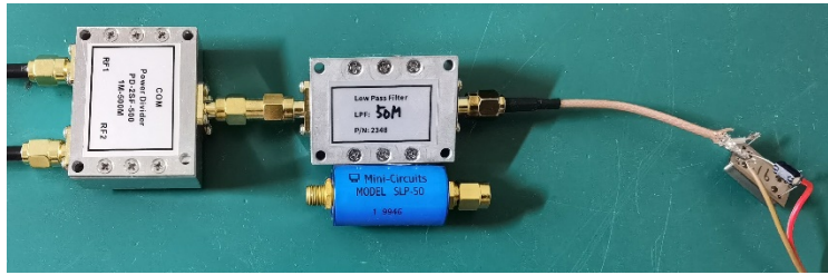
Figure 36: Test chain: splitter, low-pass filter, attenuator.
