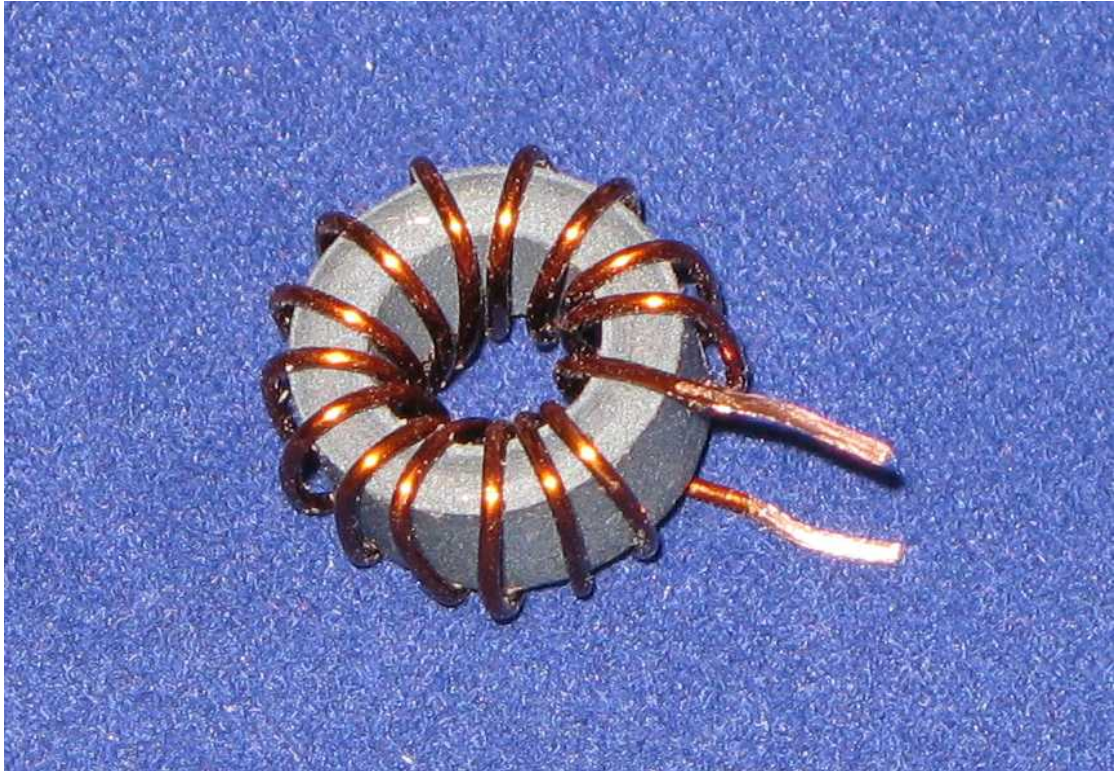
The picture shows 15 turns on NXO-100 small toroid, used for RFC. Note how I account 15 turns.
