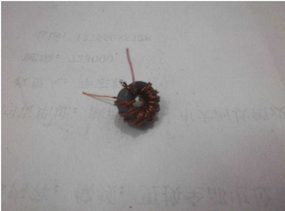
This picture shows the way to wind the bifilar coil in SWR detection circuit. Note that bifilar coils are connected end to end in the middle, and soldered.
