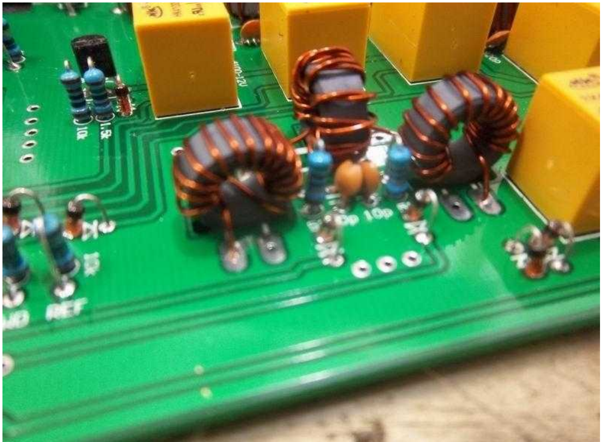
The picture shows the coils are partially soldered on the PCB. Note that different phase coils are installed but one turn is not added yet.
