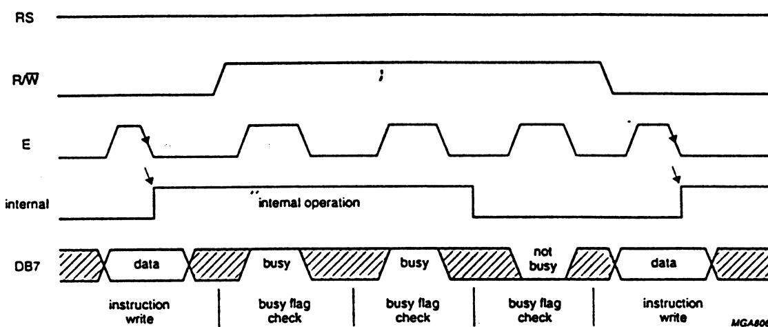
Fig.20 Example of busy flag check timing sequence.
