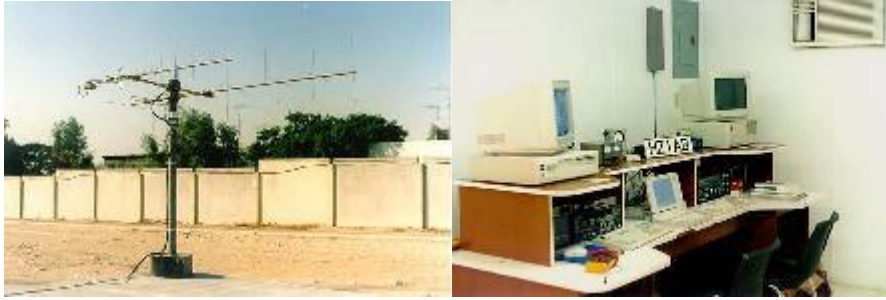
Satellite antenna and the Satellite operating position. The antenna was built by Ken/GW0RHC, Vic/KE4AQU (now KC6VAO) and Rick/KH6SAT. It was made using 1/3 of an oil drum and a 4-inch plastic pipe filled with concrete. New Shack
