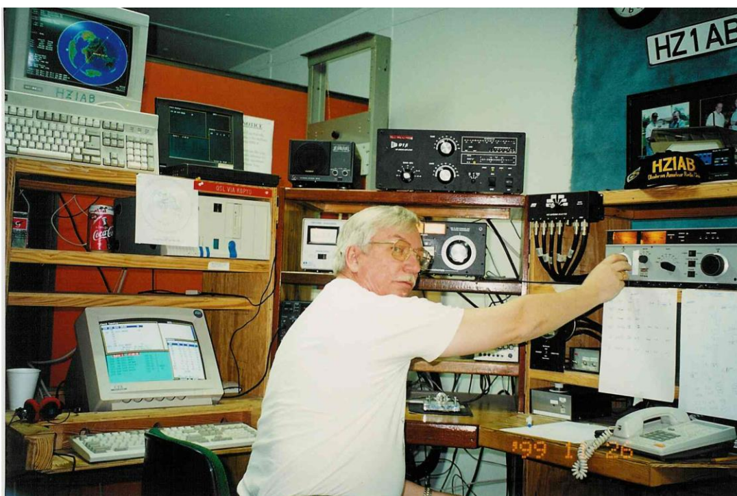
Thomas, SM0CXU. At the end, the only remaining CW Operator, and the author to this History Book. Picture from CQWW-CW 1999. Note the two pre-tuned amplifiers (TT Titan and Alpha 91b), for swift moves between the bands
