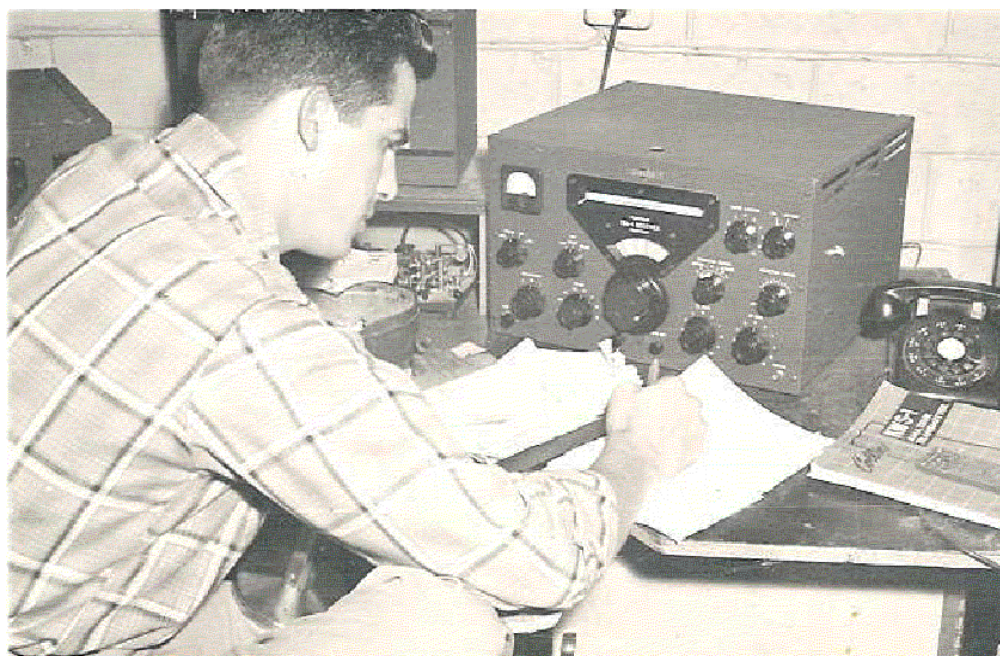
Marc, W4WM then K4LYG operating HZ1AB late 1956 or early 57. The station was Collins 75A4 and KWS1, the antenna was a sloping V-Beam out near the end of the main runway.
