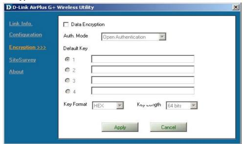
**Data Encryption** – enable Encryption by clicking on the box. Encryption is disabled as the default setting.
