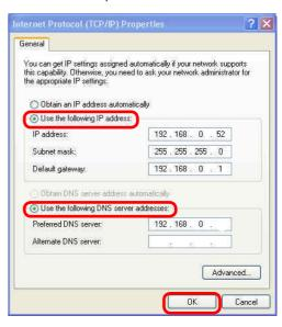
You have completed the assignment of a Static IP Address. (You do not need to assign a Static IP Address if you have a DHCP-capable Gateway/Router.) 36
