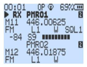
In the frequency mode you manually type in the frequency with the keypad. You can also switch different options for that VFO in the menu (first 13 menu entries). If you setup the VFO, the settings can be saved to a memory channel by going into the menu chsave and choosing the memory channel the VFO should be saved into.
