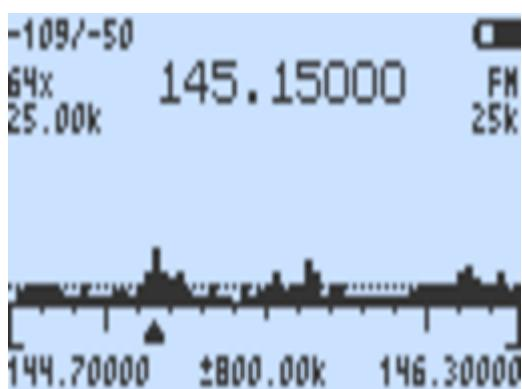
Spectrum analyzer can also be used with [ScnRng mode](#)
