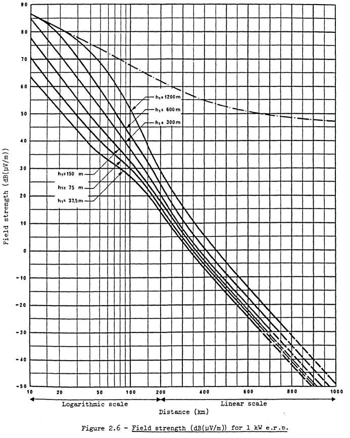
Frequency : 30 to 250 MHz; Land; 5% of the time; 50% of the locations;  $h_2 = 10 \text{ m}$ \_\_\_\_\_ Free space
