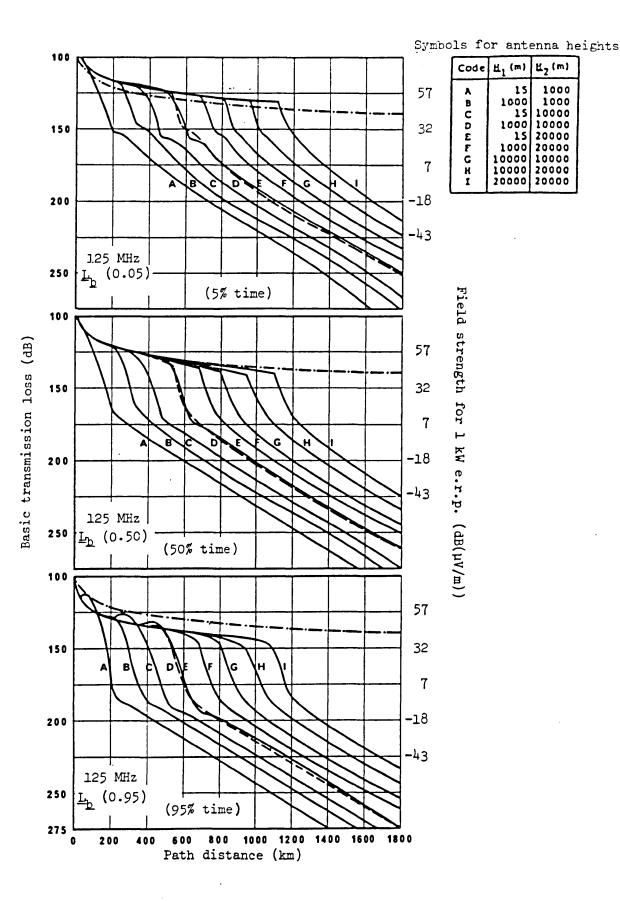
Figure 2.10 - <u>Basic transmission less at 125 MIz for 5%</u>, 50% and 95% of the time. .-... Free space
