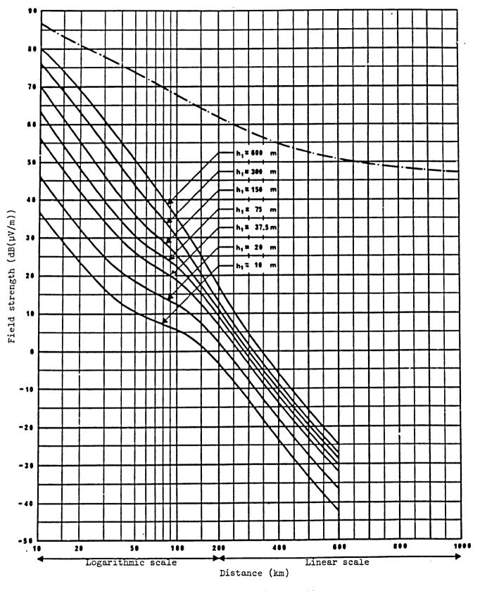
Figure 2.11 - Field strength  $(dB(\mu V/m))$  for 1 kW e.r.p.
