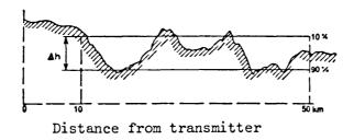
Figure 2.15 - Definition of the parameter  $\Delta h$
