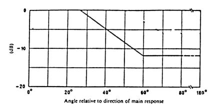
Figure 3.3 - Discrimination obtained by the use of directional receiving antennas
