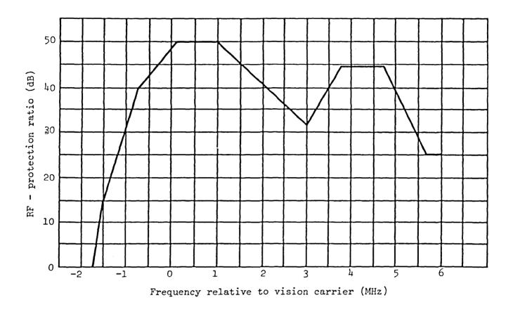
Figure 4.1 - D/SECAM television system Protection ratio in the case of frequencymodulated sound broadcasting tropospheric interference
