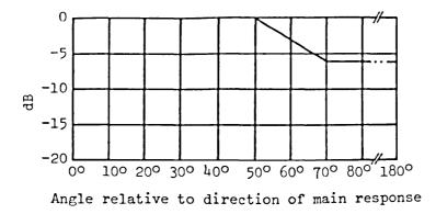
Figure 1 - <u>Discrimination obtained by the use of a directional receiving</u> <u>antenna for the television stations in the band 87.5 to 100 MHz</u>
