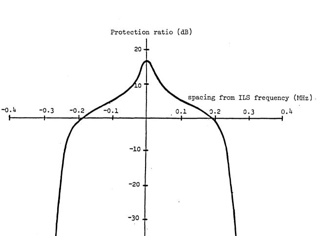
Figure 5.3 - Protection ratio for Type A 1) interference
