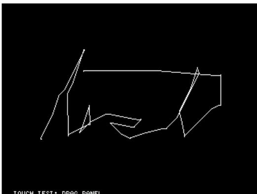
You can test the touch panel by selecting **CONFIG → TOUCH TEST**. A line is drawn while dragging the stylus along the touch panel. When released from the touch panel, it returns to its original state.
