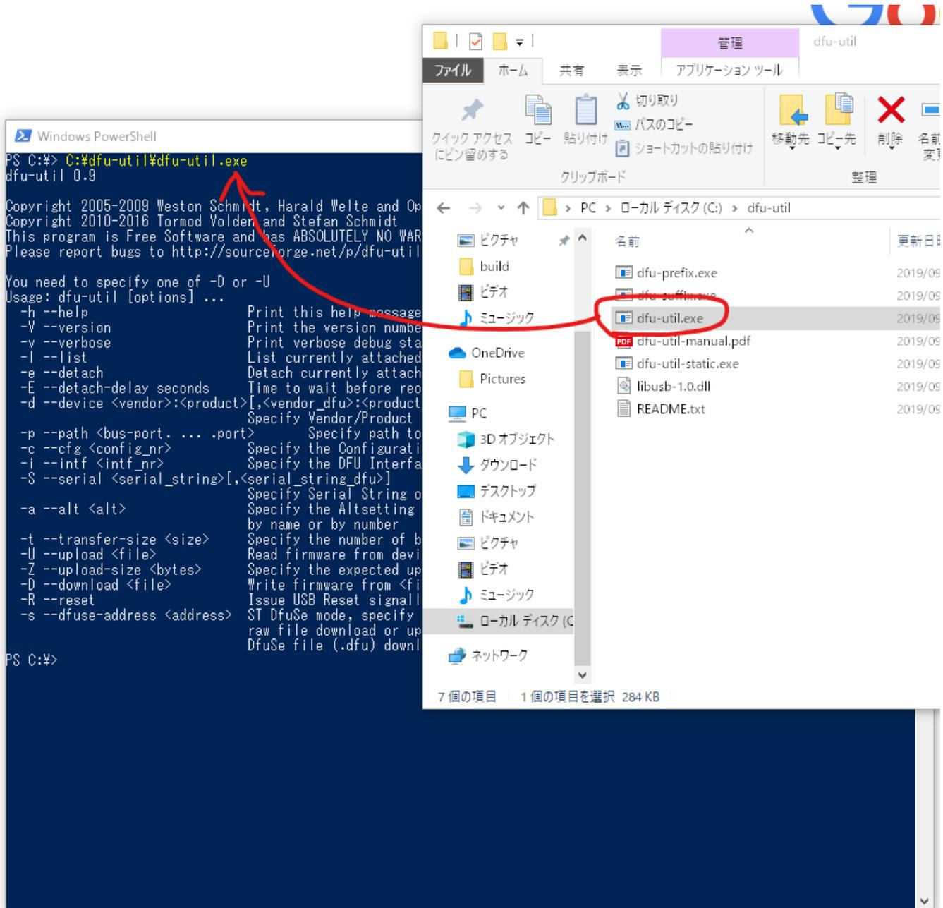
When dfu-util.exe is dragged and dropped from Windows Explorer to PowerShell, the path is automatically inserted. Dfu-util version can be displayed by starting with `--version` as follows.
