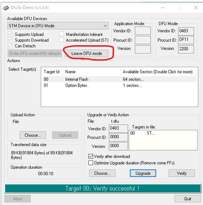
This screen will be displayed when writing is complete. Click the Leave DFU mode button to exit DFU mode. The device will reset and boot with the new firmware.
