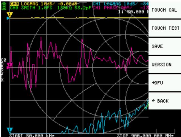
The **CONFIG** menu allows you to make general settings for the device.
