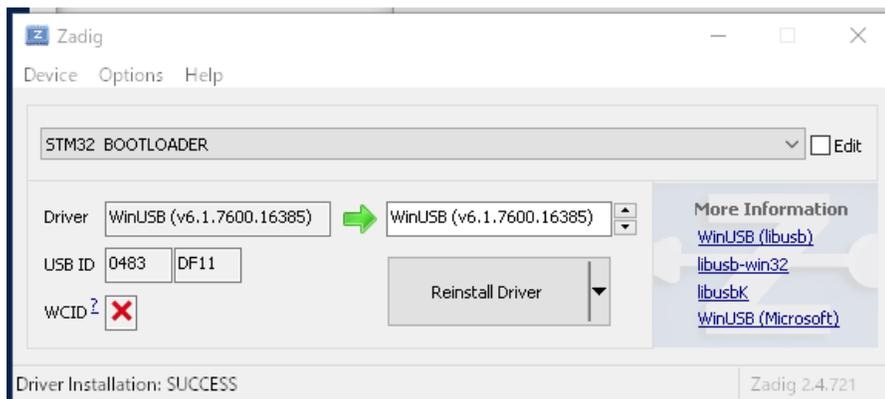
\* If you want to restore the driver, find the corresponding device from “Universal Serial Bus Controller” in “Device Manager” and execute “Uninstall Device”. The driver is automatically installed when the USB connector is disconnected and reinserted.
