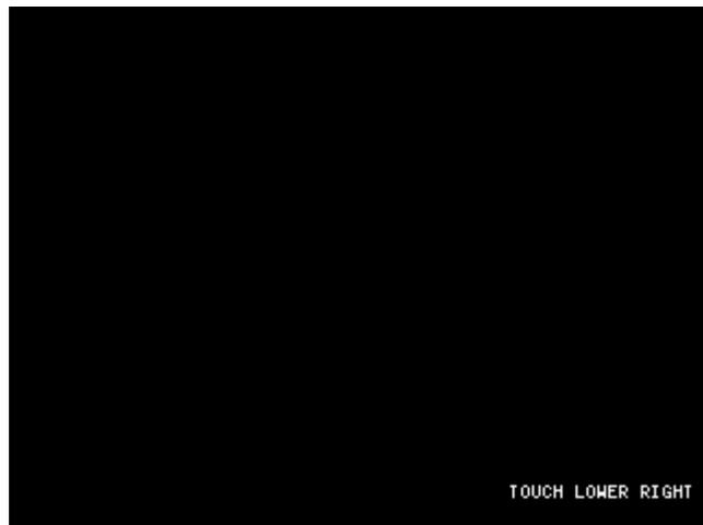
**CONFIG** → **TOUCH CAL** is selected, the touch panel can be calibrated. If there is a large difference between the actual tap position and the recognized tap position, this can be solved by executing this. After performing **TOUCH CAL**, perform **TOUCH TEST** to confirm that the settings are correct.
