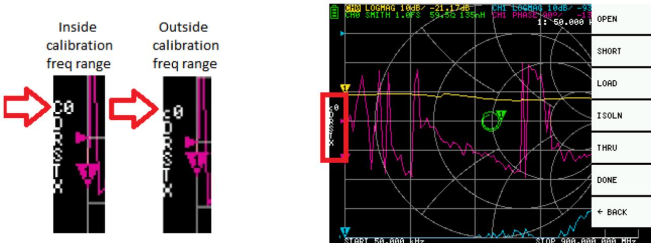
Calibration should basically be performed whenever the frequency range to be measured is changed. If the error has been corrected correctly, the calibration status display on the screen will be **Cn DRSTX** Where: **n** is the calibration dataset number being loaded.
