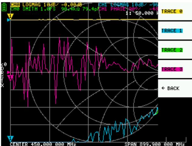
Up to four traces can be displayed, one of which is the active trace.
