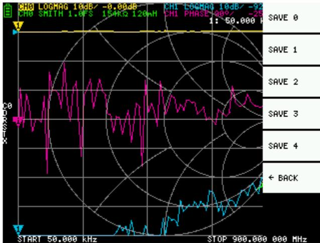
Up to 5 calibration datasets can be saved. NanoVNA loads number 0 data immediately after startup.
