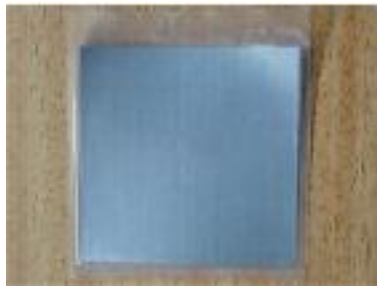
1 sq inch metal strip showing K peak with scatter
