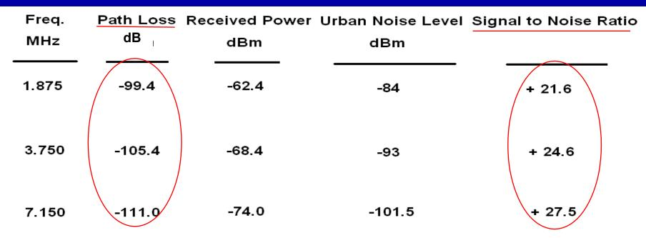
This example assumes that both the transmitting antenna and the receiving antenna are isotropic radiators with Gain = 0 dBi. Also assumed is that any transmission line losses are 0 dB at both ends of the link.
