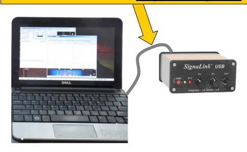
Computer does digital mode encode and decode
