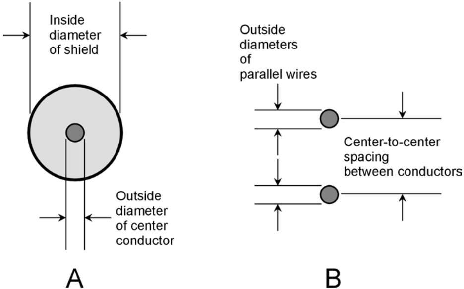
**15-8** Edge-on views of coaxial transmission line (A) and parallel-wire line (B). In either type of line,  $Z_0$  depends on the conductor diameters and spacing, and on the nature of the dielectric material between the conductors. See text for discussion.
