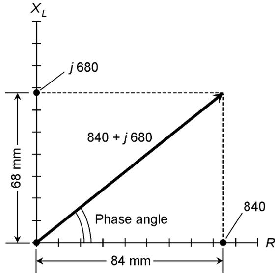
phase angle is the angle between this vector and the  $R$  axis. It will be the same as the angle of the slanted line in Fig. 13-12.
