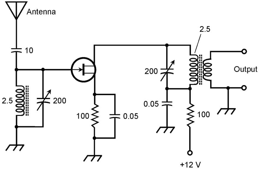
**24-9** A tuned RF amplifier for use at about 10 MHz. Resistances are in ohms. Capacitances are in microfarads ( $\mu\text{F}$ ) if less than 1, and in picofarads (pF) if more than 1. Inductances are in microhenrys ( $\mu\text{H}$ ).
