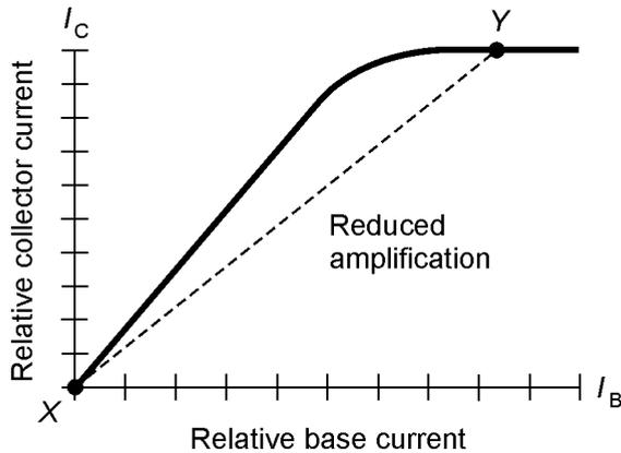
Then,  $dI_C/dI_B$  is reduced, as shown in Fig. 22-7. Points X and Y in the graph represent the instantaneous current extremes during the signal cycle in this particular case.
