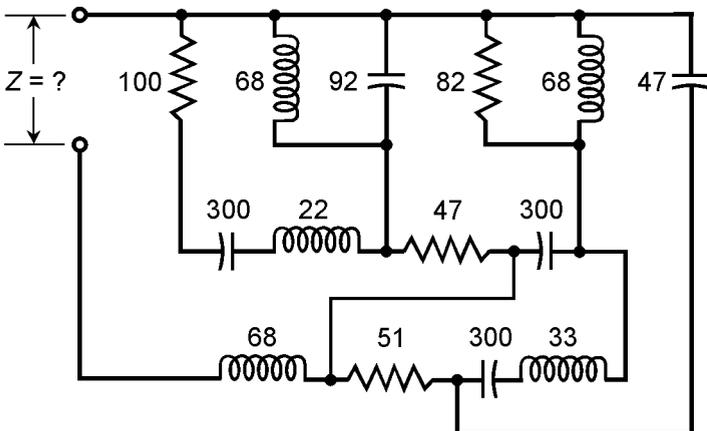
**16-10** A series-parallel nightmare circuit containing multiple resistances and reactances. Resistances are in ohms; inductances are in microhenrys ( $\mu\text{H}$ ); capacitances are in picofarads (pF).
