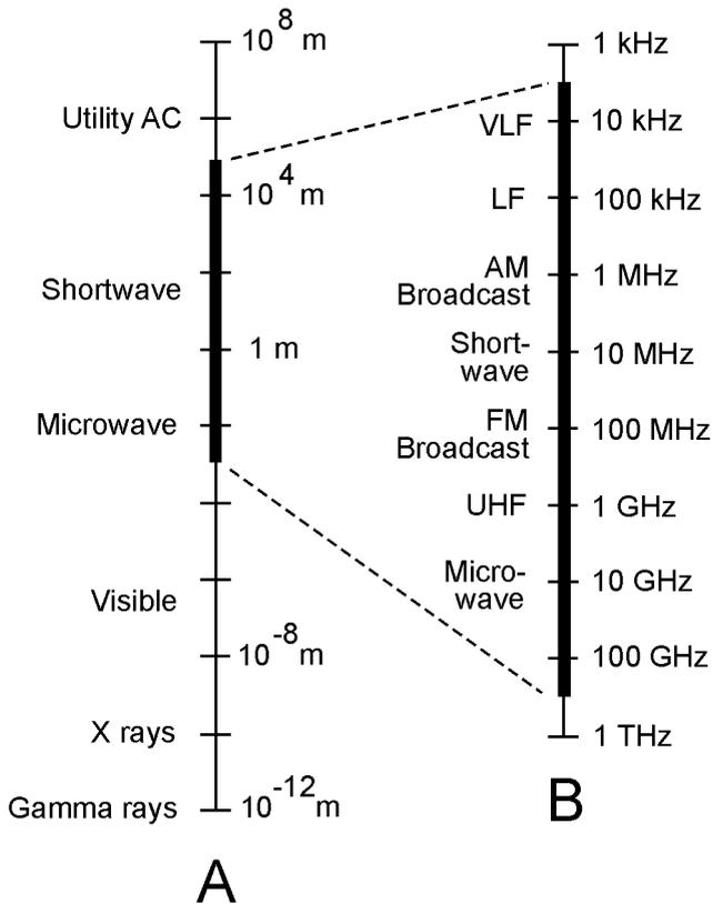
**25-10** At A, the EM spectrum from  $10^8$  m to  $10^{-12}$  m, with each vertical division representing two orders of magnitude (an increase or decrease of the wavelength by a factor of 100). At B, the RF spectrum, with each vertical division representing one order of magnitude (an increase or decrease of the frequency by a factor of 10).
