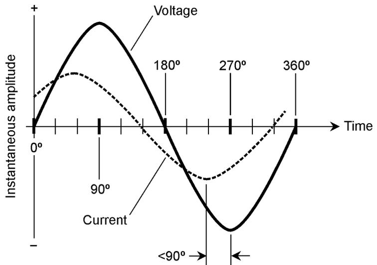
the circuit conductors. In either case, the situation can be represented by a resistance,  $R$ , in series with a capacitive reactance,  $X_C$  (Fig. 14-10).
