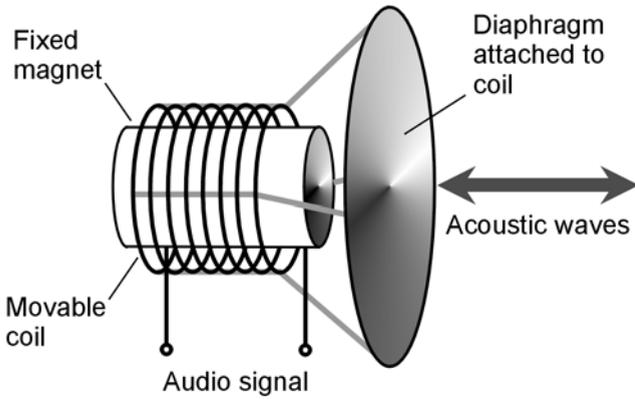
30-1 Functional diagram of a dynamic sound transducer.
