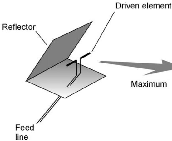
**27-13** A corner reflector with a dipole as the driven element.
