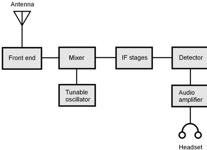
25-12 Block diagram of a single-conversion superheterodyne receiver.
