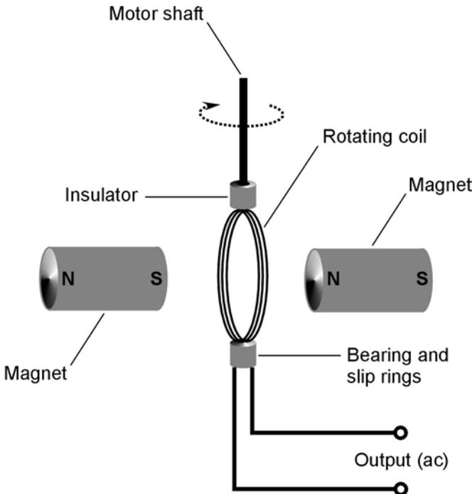
**9-14** A functional diagram of an ac generator.
