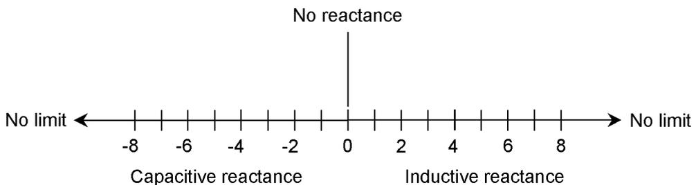
**14-1** Inductive and capacitive reactance can be represented as numerical values (corresponding to ohms multiplied by  $j$ ) along a number line.
