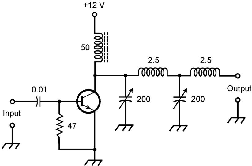
**24-11** A tuned RF power amplifier, capable of producing a few watts output. Resistances are in ohms. Capacitances are in microfarads ( $\mu\text{F}$ ) if less than 1, and in picofarads ( $\text{pF}$ ) if more than 1. Inductances are in microhenrys ( $\mu\text{H}$ ).
