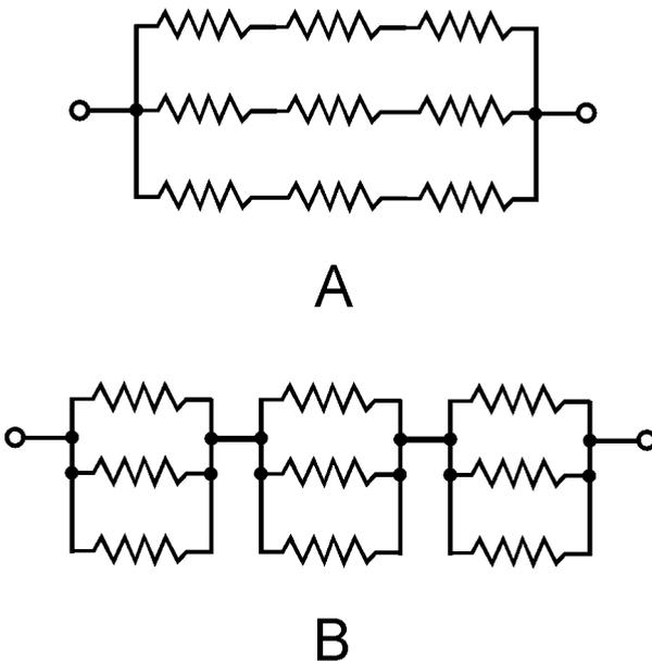
**4-10** Series-parallel resistances. At A, sets of series resistors are connected in parallel. At B, sets of parallel resistances are connected in series. These examples show symmetrical  $n$ -by- $n$  matrices with  $n = 3$ .
