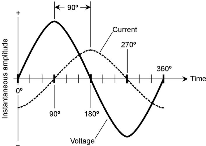
**13-8** In a pure inductive reactance, the current lags the voltage by 90°.
