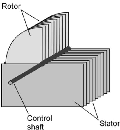
**11-8** A simplified drawing of an air-variable capacitor.
