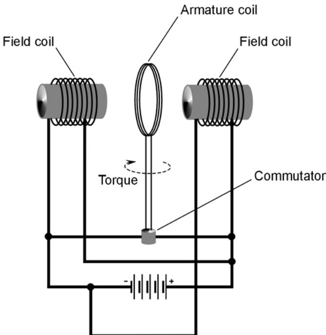
8-9 A functional diagram of a dc motor.
