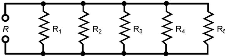
4-9 Five resistors of values  $R_1$  through  $R_5$ , connected in parallel, produce a net resistance  $R$ . Illustration for Problems 4-15 and 4-16.
