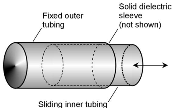
Coaxial capacitors are used in RF applications, particularly in antenna systems. Their values are generally from a few picofarads up to about 100 pF.
