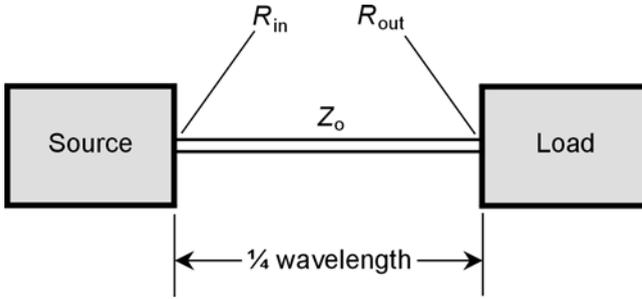
**18-11** A quarter-wave matching section of transmission line. The input impedance is  $R_{in}$ , the output impedance is  $R_{out}$ , and the characteristic impedance of the line is  $Z_o$ .
