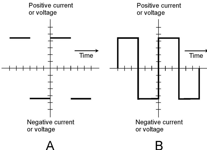
**9-2** At A, a perfect square wave; the transitions are instantaneous and therefore do not show up on the graph. At B, the more common rendition of a square wave, showing the transitions as vertical lines.
