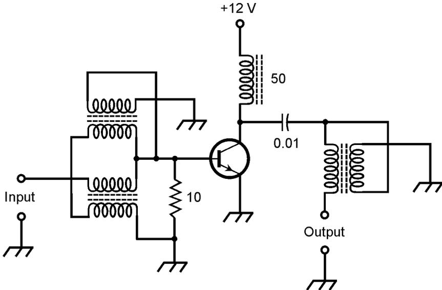
**24-10** A broadband RF power amplifier, capable of producing a few watts output. Resistances are in ohms. Capacitances are in microfarads ( $\mu\text{F}$ ). Inductances are in microhenrys ( $\mu\text{H}$ ).
