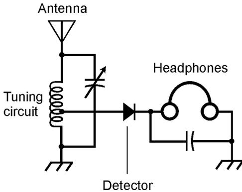
**20-2** Schematic diagram of a crystal-set radio receiver.
