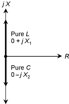
**16-1** Pure inductance and pure capacitance are represented by reactance vectors that point straight up and down.
