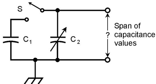
42. In Fig. Exam-2, suppose the value of the fixed capacitor,  $C_1$ , is 330 pF, and the range of the variable capacitor,  $C_2$ , is 10 to 365 pF. What is the span of capacitance values (minimum to maximum) that can be obtained with this parallel combination, with switch S either open or closed, as desired?
