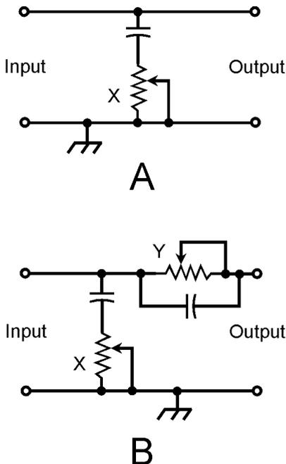
**31-3** Methods of tone control. At A, a single potentiometer/capacitor combination (X) provides treble attenuation only. At B, one potentiometer/capacitor combination (X) attenuates the treble, and the other (Y) attenuates the bass.
