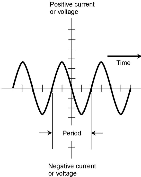
**9-1** A sine wave. The period is the length of time it takes for one cycle to be completed.
