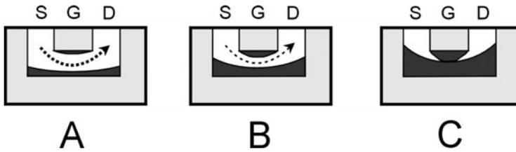
**23-3** At A, the depletion region (darkest area) is narrow, the channel (white area) is wide, and many charge carriers (heavy dashed line) flow. At B, the depletion region is wider, the channel is narrower, and fewer charge carriers flow. At C, the depletion region obstructs the channel, and no charge carriers flow.
