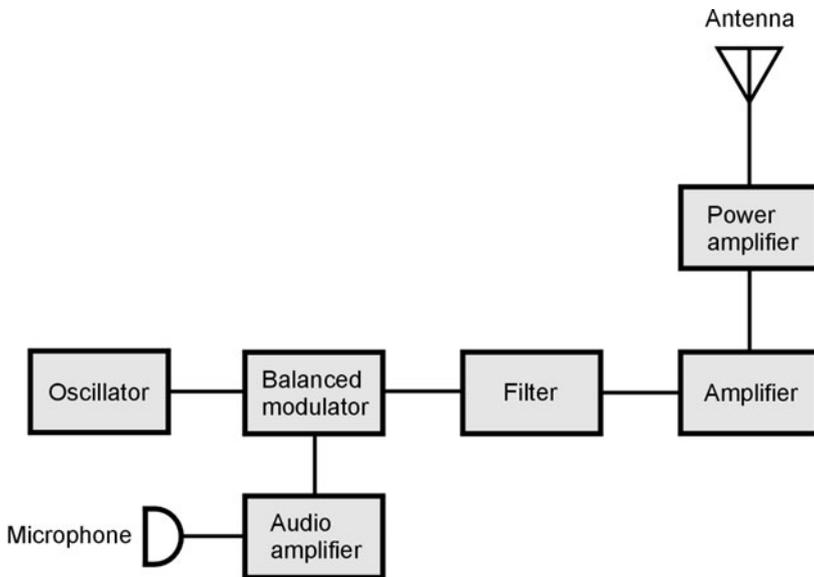
**25-6** Block diagram of a basic SSB transmitter.
