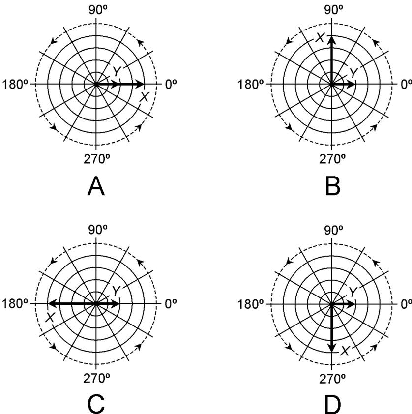
**12-11** Vector representations of phase difference. At A, waves  $X$  and  $Y$  are in phase. At B,  $X$  leads  $Y$  by  $90^\circ$ . At C,  $X$  and  $Y$  are  $180^\circ$  out of phase. At D,  $X$  lags  $Y$  by  $90^\circ$ . Time is represented by counterclockwise motion of both vectors at a constant angular speed.
