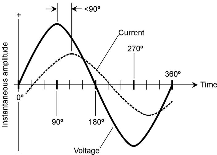
**13-9** In a circuit with inductive reactance and resistance, the current lags the voltage by less than 90°.
