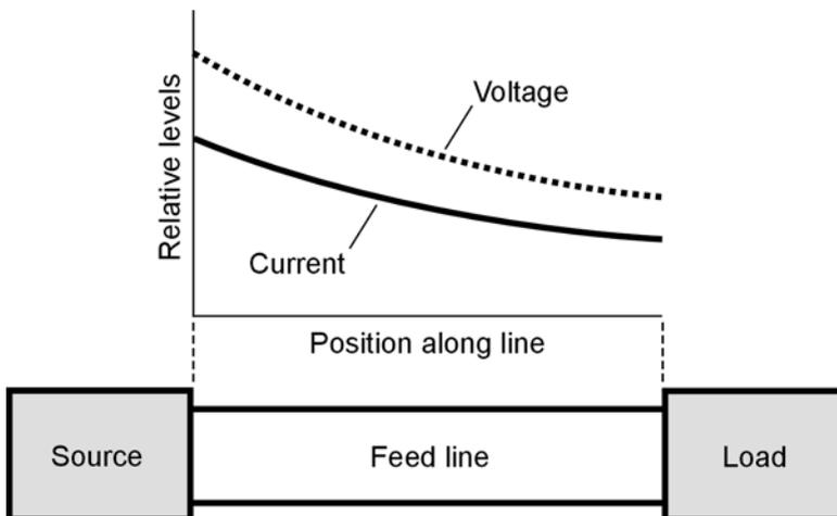
**17-10** In a matched line, the ratio of the voltage to the current ( $E/I$ ) is constant everywhere along the line, although the actual values of  $E$  and  $I$  decrease with increasing distance from the source.
