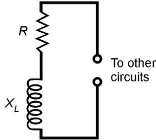
decreases until it is comparable to the loss resistance  $R$  in the coil winding. In either case, the situation can be schematically represented by an inductance in series with a resistance (Fig. 13-10).
