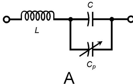
**17-13** Padding capacitors ( $C_p$ ) allow limited adjustment of the resonant frequency in a series  $LC$  circuit (as shown at A), or in a parallel  $LC$  circuit (as shown at B).
