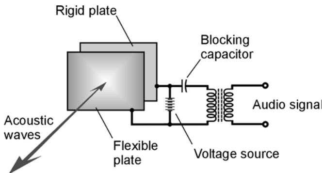
30-2 Functional diagram of an electrostatic sound transducer.
