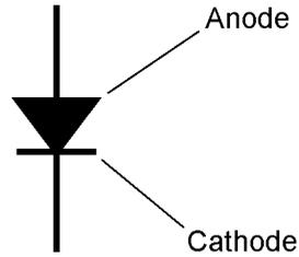
In the diode as shown in Figure 19-3, electrons can move easily in the direction opposite the arrow, and holes can move easily in the direction in which the arrow points. But current cannot, under most conditions, flow the other way. Electrons normally do not move with the arrow, and holes normally do not move against the arrow.
