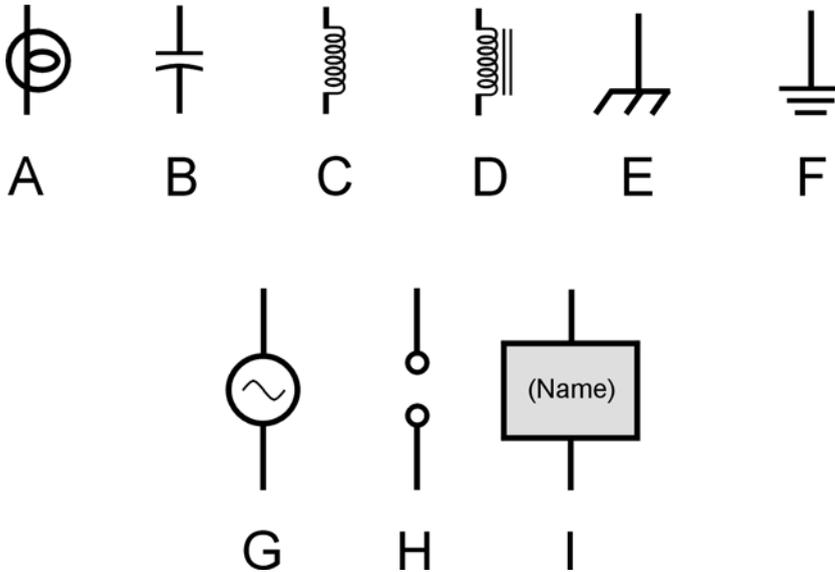
**4-4** Schematic symbols for incandescent lamp (A), fixed capacitor (B), fixed inductor with air core (C), fixed inductor with laminated-iron core (D), chassis ground (E), earth ground (F), signal generator or source of alternating current (G), pair of terminals (H), and specialized component or device (I).
