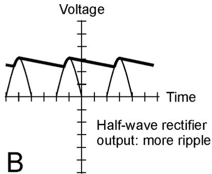
21-6 At A, a capacitor-input filter. At B, a choke-input filter.
