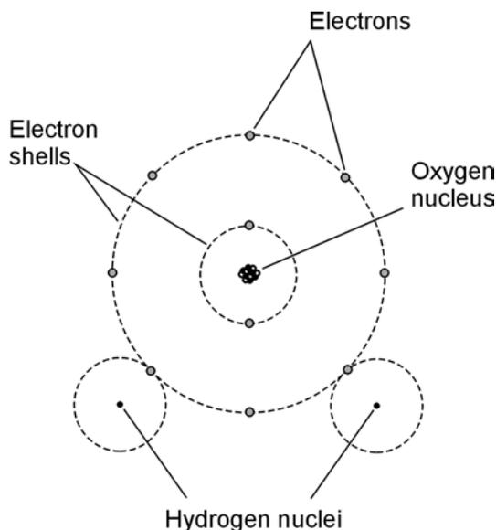
**1-3** A simplified diagram of a water molecule.
