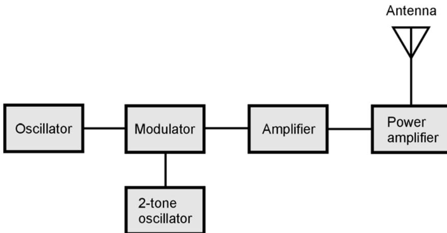
25-1 Simplified block diagram of an AFSK transmitter.
