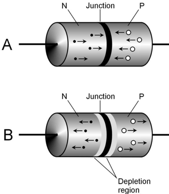
**19-5** At A, forward bias of a P-N junction. At B, reverse bias of the same junction. Solid black dots represent electrons. White dots represent holes. Arrows indicate direction of charge-carrier movement.
