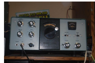
Lou's HF transceiver, the venerable Heathkit, HW-101.
