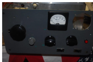
KC9YFU is currently working on building a home-brew HF amplifier using two 4-400 A tubes.
