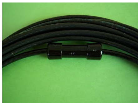
Close up of the epoxy cpvc tube over the shorting point.
