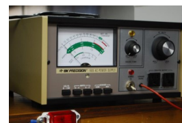
Tim's all-in-one isolation transformer and variac in one convenient box.
