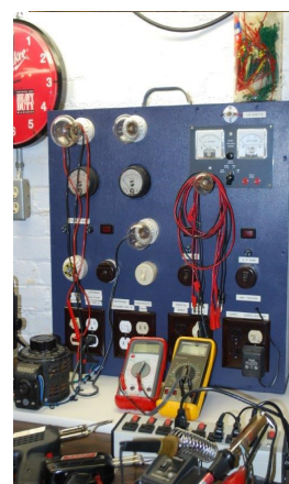
KC9HQA's home-brewed fused power distribution panel for working on radio equipment. Notice the variac on the left for safely varying volt-
