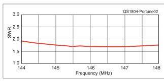
Figure 2 — The SWR of the coat hanger vertical is less than 2 across the 2-meter band.
