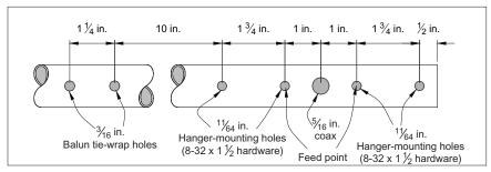
**Figure 3** — Nominal positions of holes to be drilled on the PVC mast. The hanger-mounting holes may have to be shifted slightly to accommodate tuning.
