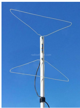
2 meter vertical antenna built with coat hangers
