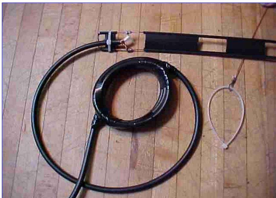
This decoupling loop is sometimes mistaken for a matching balun.
