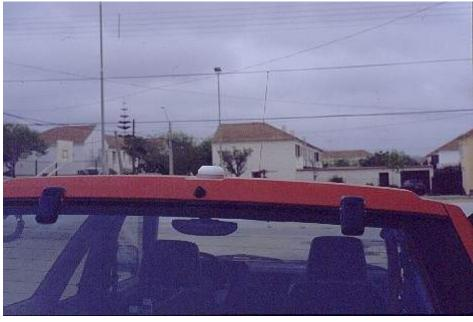
When the antenna is dismounted, a simple cap is screwed onto the base, in order to protect the contacts from dirt, water and corrosion. This is how the car roof looks with dismounted antenna. Only the quarter wave whip for VHF remains in place at all times, since it fits easily into most garages. The other wires in this photo are power and phone lines in the background!
