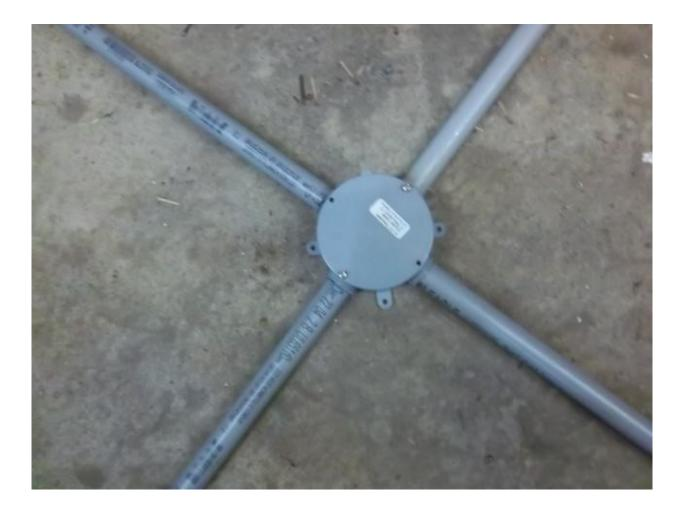
The antenna is constructed using a 4-way electrical conduit junction box and 3/4" PVC electrical conduit as shown above.
