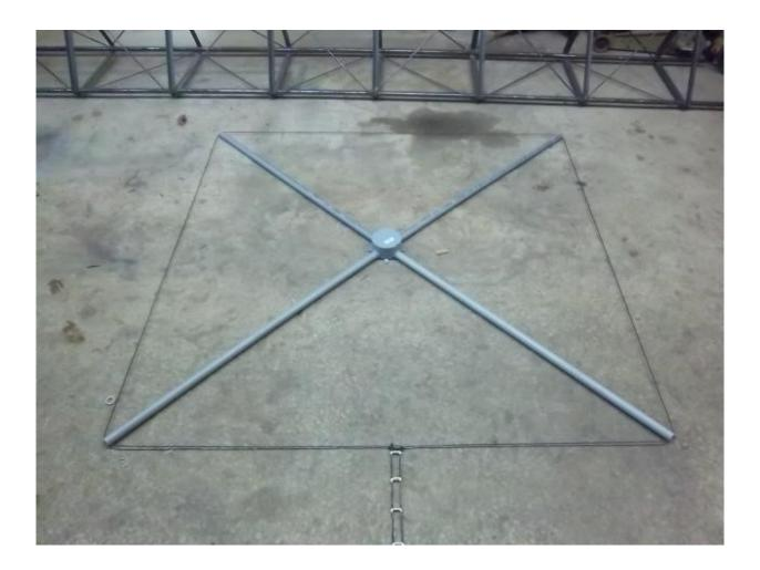
The length of a full-wave antenna is given by the formula 1005 / frequency in MHz = total length of the loop.
