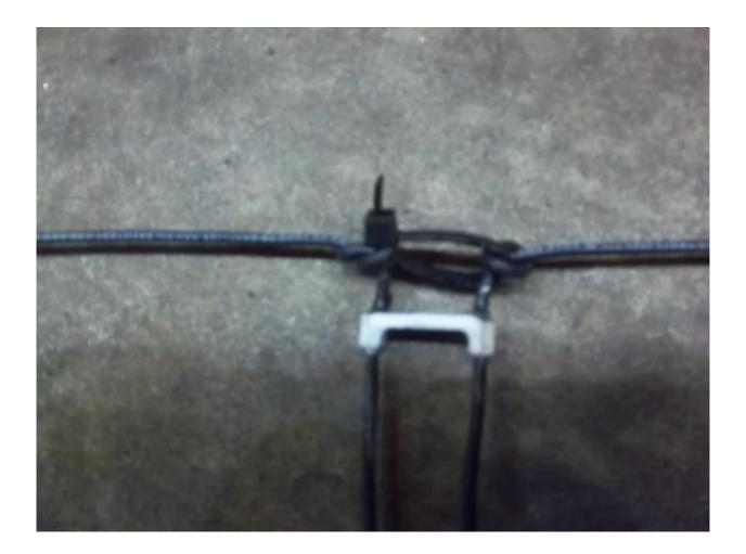
This photo shows the detail of how I made the a parallel feeder stub integral with the loop antenna. Simply tie an overhand knot in the loop ends, use a plastic tie to tension the wire on the spreaders, and place a feedline spreader close to the junction to keep it tight.
