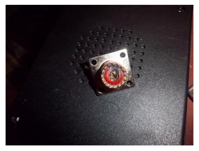
A burned out SO-239 from a balun that arc'd over at about 2,000 volts from a linear power amplifier feeding an antenna at high SWR. Keep in mind that SWR on the feedline and antenna with parallel-feedline DOES NOT MATTER! All you have to do is make your
