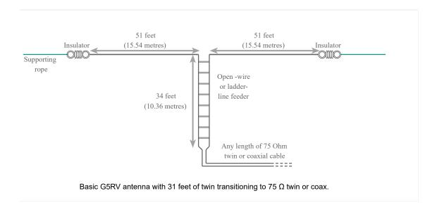
the G5RV antenna with 31 feet / 10.36 metres of open wire before transitioning to twin or coax is a nt option, another solution is to use an antenna tuning unit.
