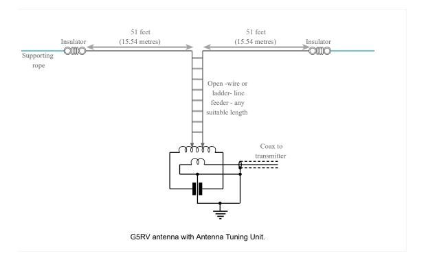
nna tuning matching unit provides two functions. One is to match the impedance because. Like any antenna, give an exact match. The second is to provide the balanced to unbalanced transition.
