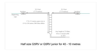
me way that the both sides of the feeder can be strapped together and the whole normal size G5RV antenna 1 a good ATU to provide coverage of 160 metres (Top Band), so too the same technique can be used with ized G5RV antenna to provide 80 metre coverage.
