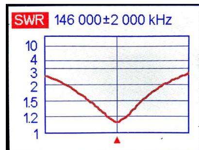
Figure 4: SWR 144-148 MHz, measured with a Rig Expert A1400.
