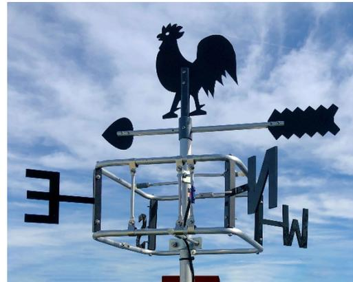
Figure 1: Concealed 2m antenna. The Rooster-Tenna
