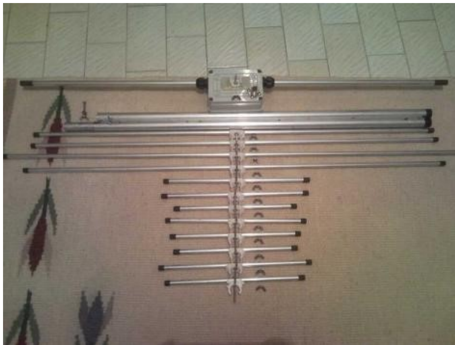
The 5-/8-Element-Duoband-Yagi as portabel version, built by Gökhan , 7
