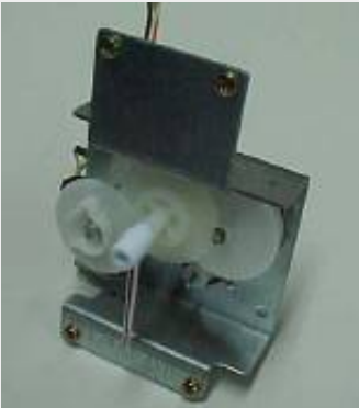
Photo 3: Mechanical indicator needle system
