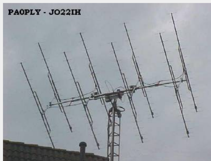
Photo 1.: Large EME array for 432MHz.
