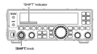
Referring to Figure "**A**", note the depiction of the IF DSP filter as the thick line, with the [**SHIFT**] knob in the 12 o'clock position. In Figure "**B**", an interfering signal has appeared inside the original passband. In Figure "**C**", you can see the effect of rotating the [**SHIFT**] knob to reduce the interference level by moving the filter passband so that the interference is outside of the passband.
