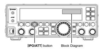
**Note** An attenuator is always "ON" between 30kHz and 1.7MHz.
