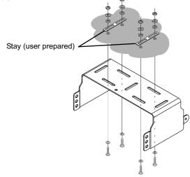
Position the transceiver in the bracket so the holes in the side are aligned with those in the bracket. Fasten the transceiver into place using the supplied Knob-screws (M4).
