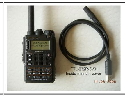
The **VX-8G** data cable is a simple wire connection at RS232 levels - no level converter. Then use a USB/serial adapter if you do not have a serial port on your PC.
