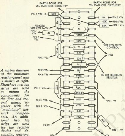
of the miniature resistor-panel unit is shown at right. Elsewhere two tag strips are used mount the components for the first and second stages, together with the 'modulator" network compon-An additents. ional two tag strips are used for the rectifier diodes and decoupling resistors.
