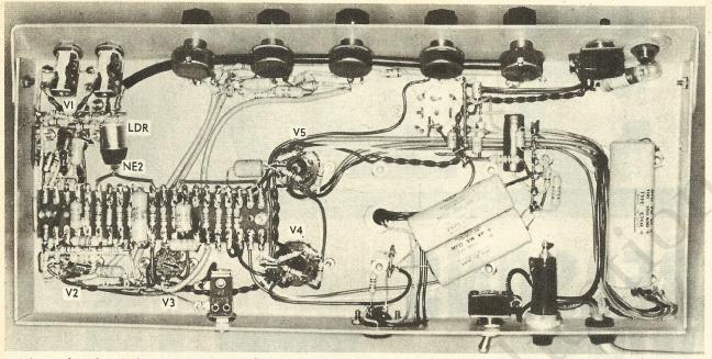
The underside of the new guitar amplisier has space to spare, apart from the "busy" area around the low-level stages. Along the rear lip of the chassis is a jack for vibrato foot control, the loudspeaker socket, mains switch and mains fuse. At the time the photograph was taken we had not installed the clip to secure the mains lead.
