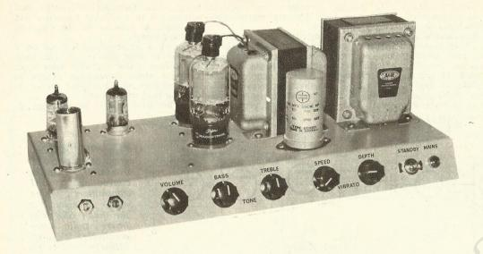
The preamplifier is in the left foreground, followed logically by other valves providing vibrato. voltage amplification and phase splitting to the two 6DQ6A output valves.
