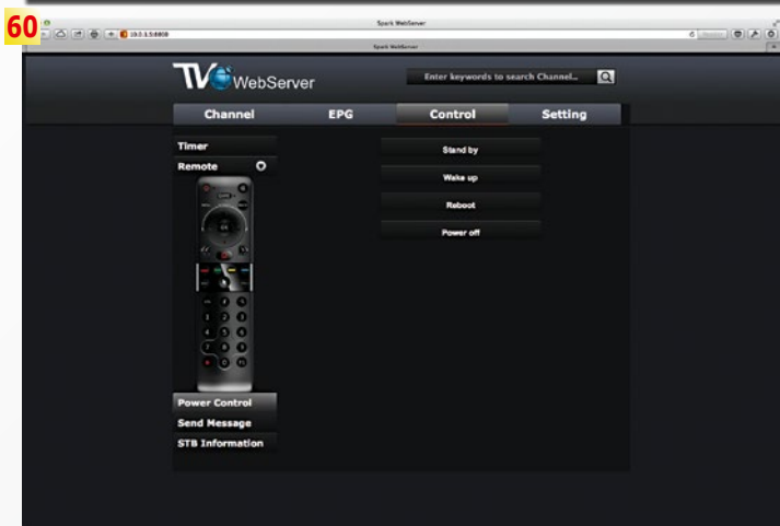
57. Web server of the Amiko A3 with live streaming of the currently received TV channel
