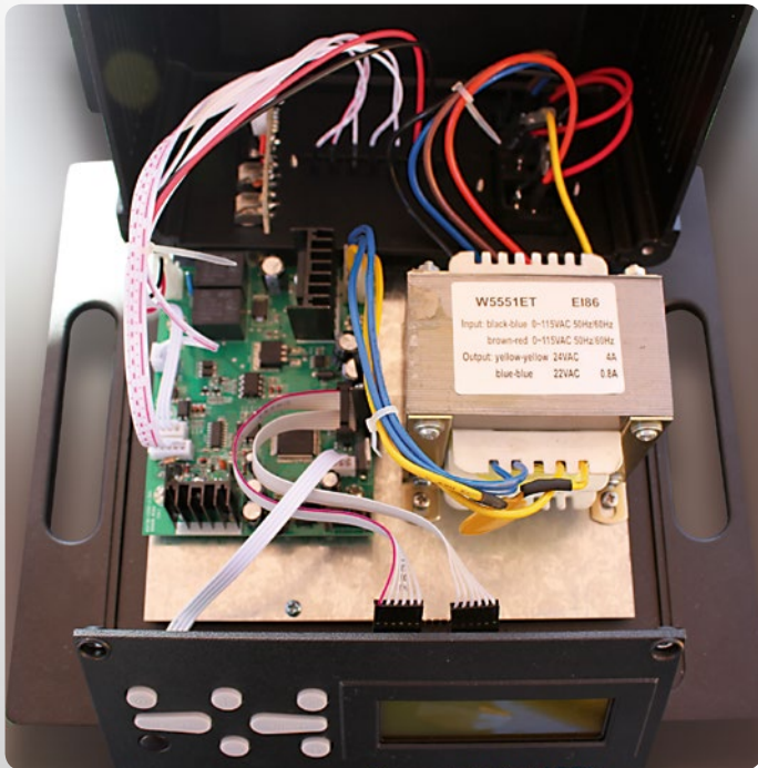
■ The Titanium ASC1 is very heavy, so what's inside? A huge transformer that will drive the biggest dish thanks to its 5 amp output. We also found exceptionally well designed PCBs with professional cables. Everything is assembled with great care. Thumbs up to Titanium for excellent workmanship!
