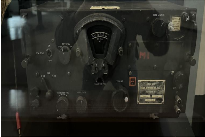
A BC-348-R receiver from a B-17 at the Mighty 8 th Air Force Museum in Pooler, GA.
