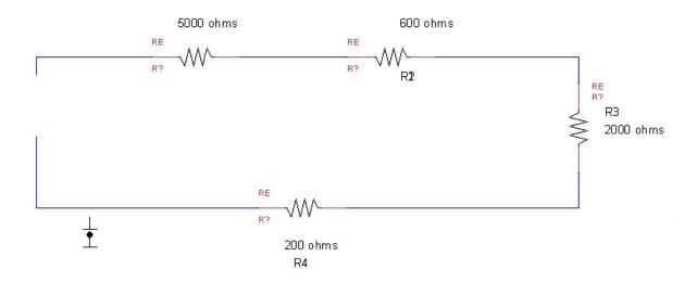
Resistance Total in a DC circuit is R1 + R2 + R3 + R4
