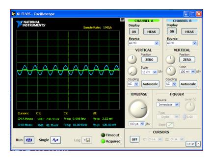
The measured gain is then  $128 \text{mV}_{pp}/2.53 \text{mV}_{pp} = 50.59 \text{V/V}$ , and similarly for the  $5 \text{mV}_{pp}$  signal. This is quite good, considering the specified voltage gain needed to be 50 V/V. The measured value is only 1.17% off of specification.
