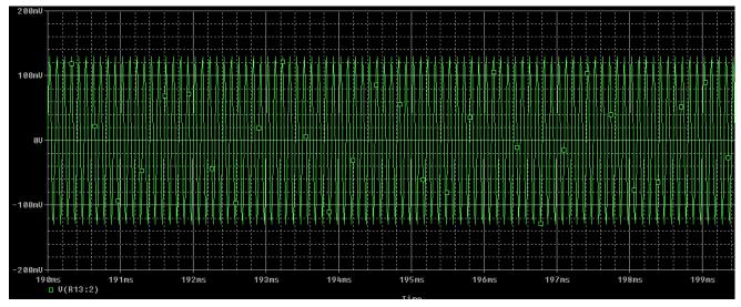
It was found in further transient simulations that the amplifier behaved properly for input signals up to 6mV, putting it safely within the design constraint of a 5mV maximum input.
