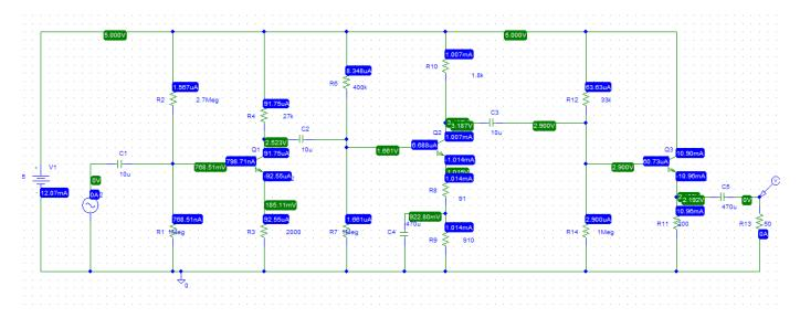
Running an AC analysis reveals the transfer function of the circuit. This amplifier will operate with 34dB (about 50V/V) of gain in the passband. The low corner frequency is at just under 10Hz and the high frequency corner is at around 100kHz, so that the amplifier will operate appropriately in the audio region.
